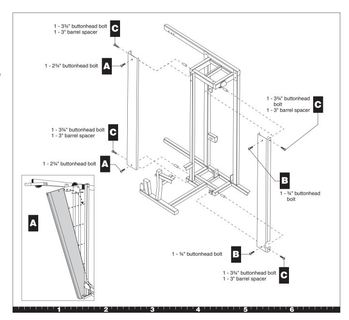
D. Attach the Side Shrouds to the Side Bracket and Main Base using four 3¾-inch buttonhead bolts four barrel spacers
